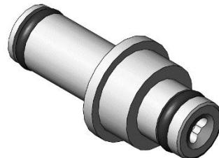
Next install two new o-rings by slipping them over both ends of the chuck tube.
